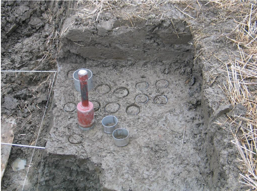
Figure 3. Sampling of small soil cores (5 cm height, 7.2 cm diameter) in field plots.
