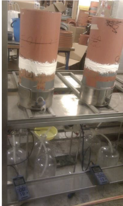
Figure 5. Equipment used for breakthrough experiments under ponding conditions on soil columns from the Lower site (Paper I).
