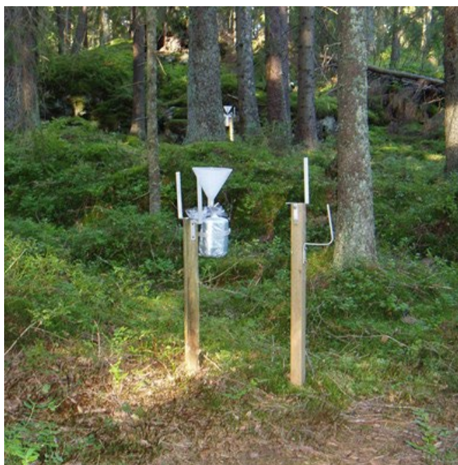
FIGURE 7.3.1. AN EXAMPLE OF A SUITABLE COLLECTOR FOR SAMPLING DEPOSITION
