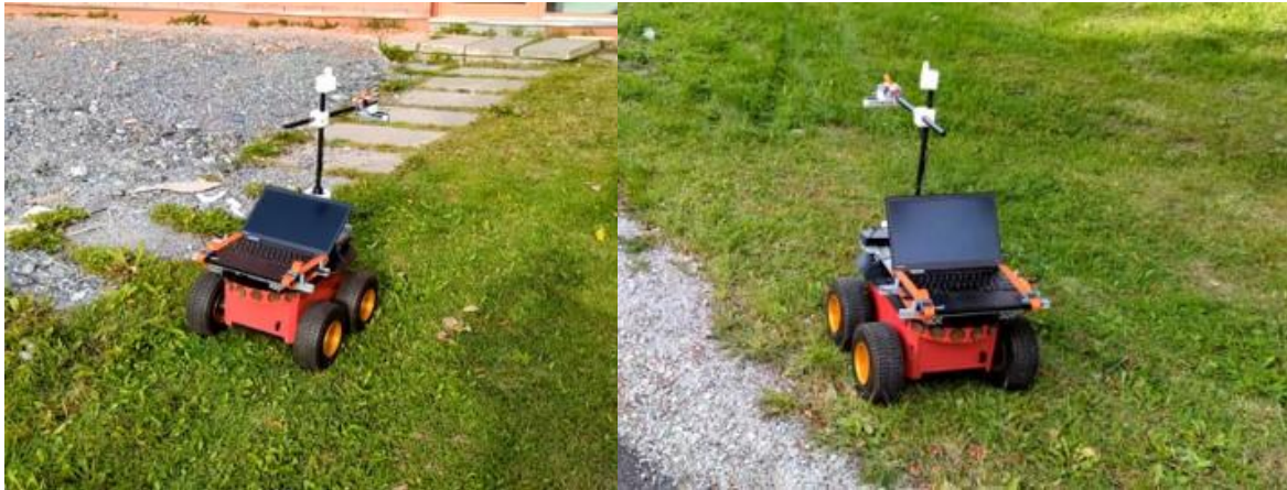
Figure 7. First pilot trial at LTU campus where we tested the sensor payload on a grassed area with and without slope. During this test the operation station was placed on the robot.
