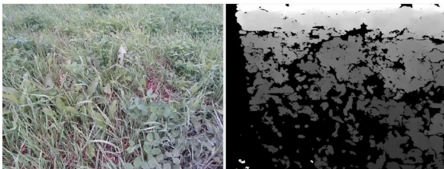
Figure 14. An example of a RGB (left) and a depth (right) image acquired by the RGB-D camera with a viewing angle of 45°.
