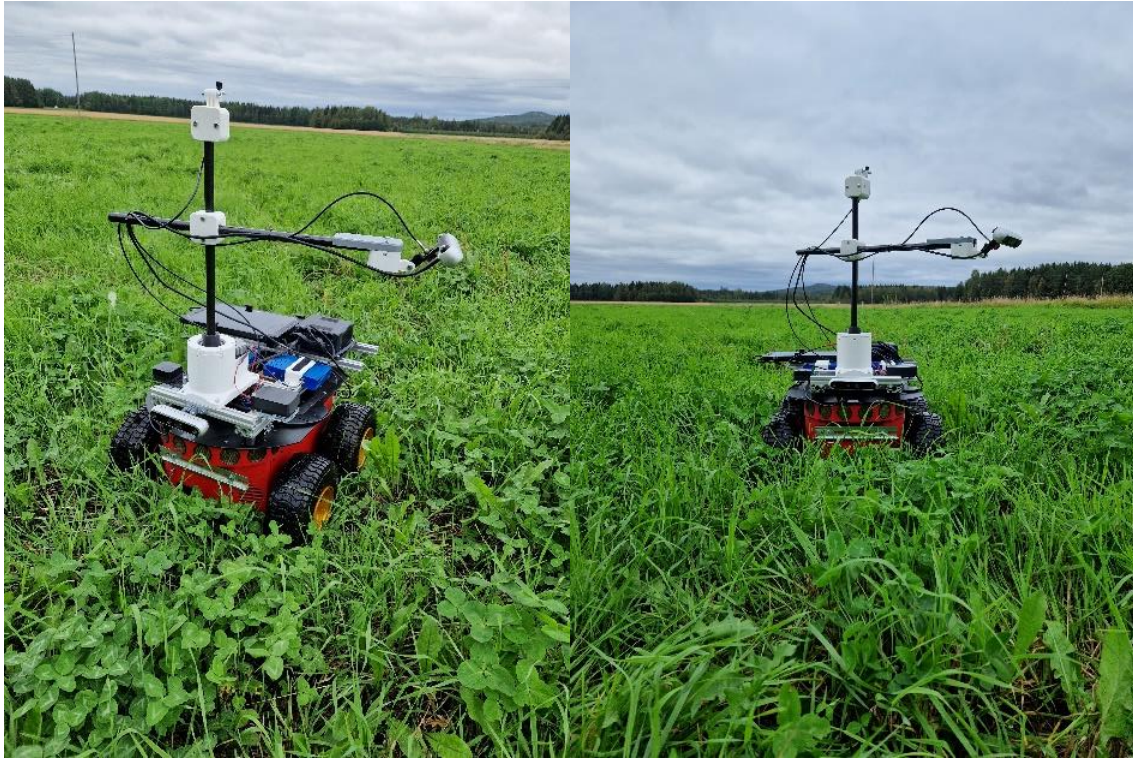
Figure 12. Perspective view of the robot in the field with the top camera (superior rod) rotating in the static position (left) and a frontal view of the robot (right).
