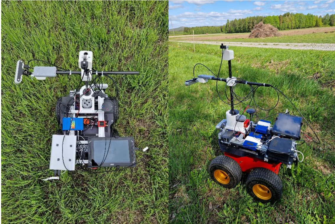
Figure 11. Top view of the robot in the field with the top camera (superior rod) in the side position (left) and a perspective view of the robot showing the top camera in front of it (right).
